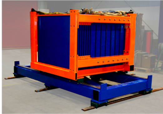
FIGURE 1.17: shows a picture of the TCMT in an orange frame on top of its support structure [81].
