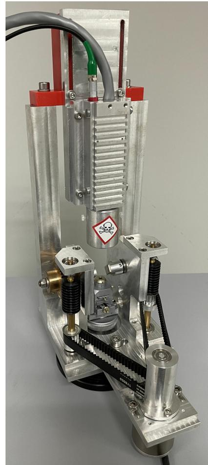
Figure D.2: The photo of the first version of the the permanent magnet system.
