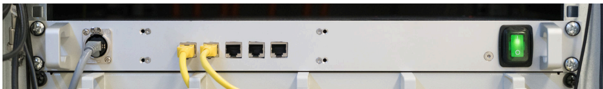
Figure 5.17: Main controlling board in the rack. The grey cable in the left is the local network connection, the five RJ-45 sockets are for the satellite connectors. The case contains a 24 V, 75 W power supply, a Raspberry Pi and a circuit board.
