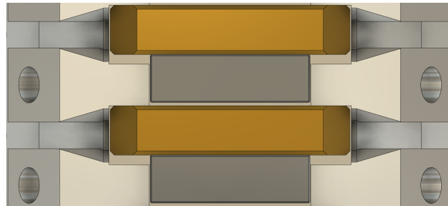
Figure 4.22 – Top view onto the girder with the magnets in yellow and the poles in dark grey. They are kept in position with the comb structure on the left and right.
