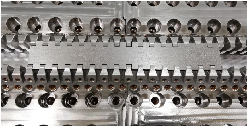
Figure 5.3 – A close up onto the alignment tool inserted into the comb structure of one girder. The increased gap for the tooth at the intersection comes from a machining error of the tool and not from the combs.
