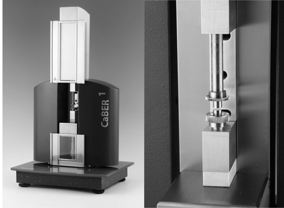
Figure 19: Front view of the capillary break-up elongational rheometer (CaBER) and the endplates between which the actual stretching takes place.
