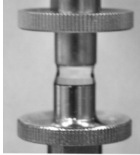
Figure 20: „Sagging“ fluid cylinder in the CaBER for Bo \gg 1 .
