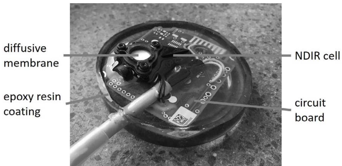
Fig. 22. Photo of the K33SOIL. The circuit board of the sensor module K33 has an area of 51 mm x 57 mm. We covered it with epoxy resin. The measuring NDIR cell is located below the diffusive membrane, which is the only part not covered in epoxy resin.
