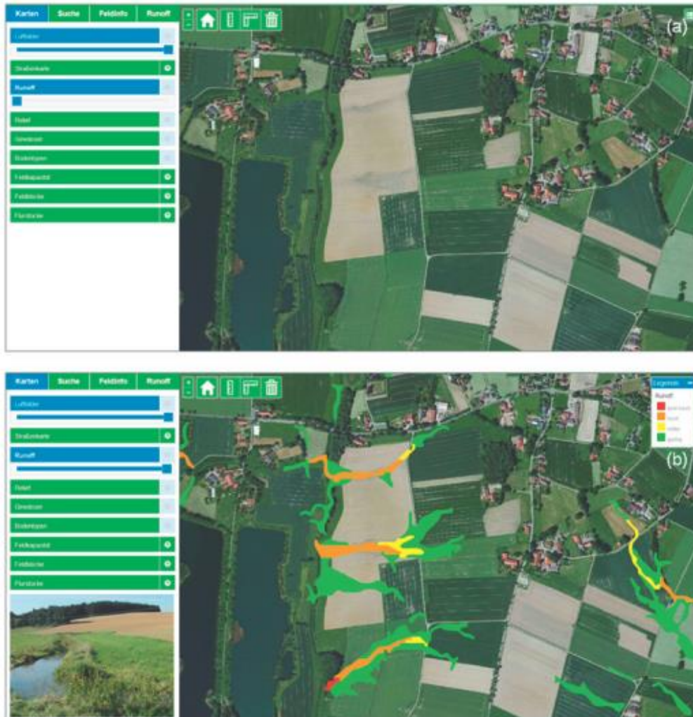
Fig. 6: Graphical user interface of the WebGIS tool 'Gewässerschutzberater' with examples for mapping applications, showing a section of the Gehle catchment in Google Earth (Fig. 6a) and the respective discrete runoff risk classes (Fig. 6b).
